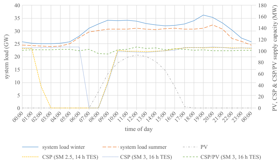
Fig. 12. Typical system load in South Africa in July (winter) and January (summer) and PV, CSP & CSP/PV supply capacity.
